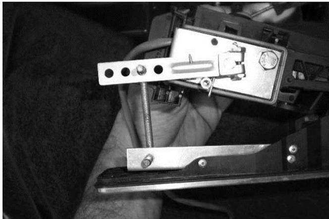
**Gambar 10.16** Potensiometer Throttle Porsche Elektrik
