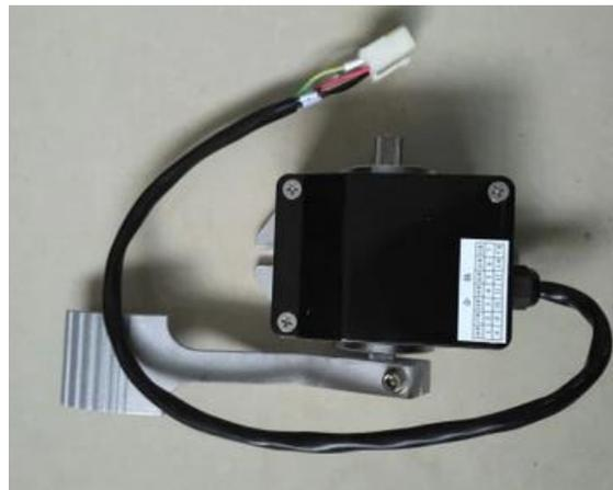
**Gambar 9.9** Potensiometer throttle pedal akselerator pengganti Curtis.
